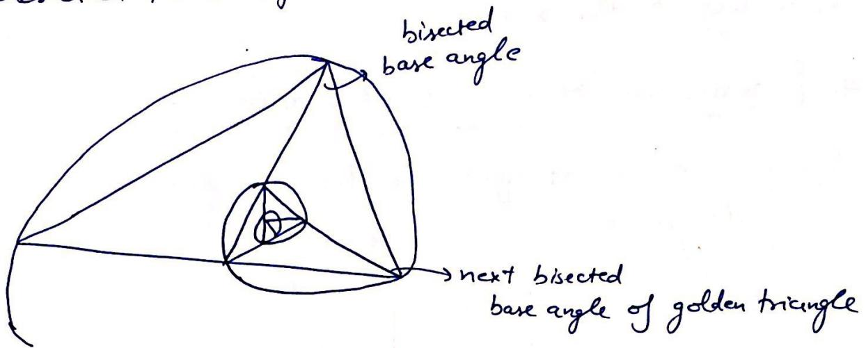
Using this method, new golden triangles may be generated here, we obtain an equiangular or logarithmic spiral in the above generated triangles. (having  $\varphi$ )
